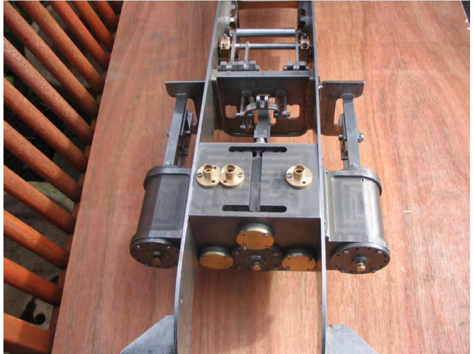
Steam fittings and Exhaust passages on the inside cylinder block
