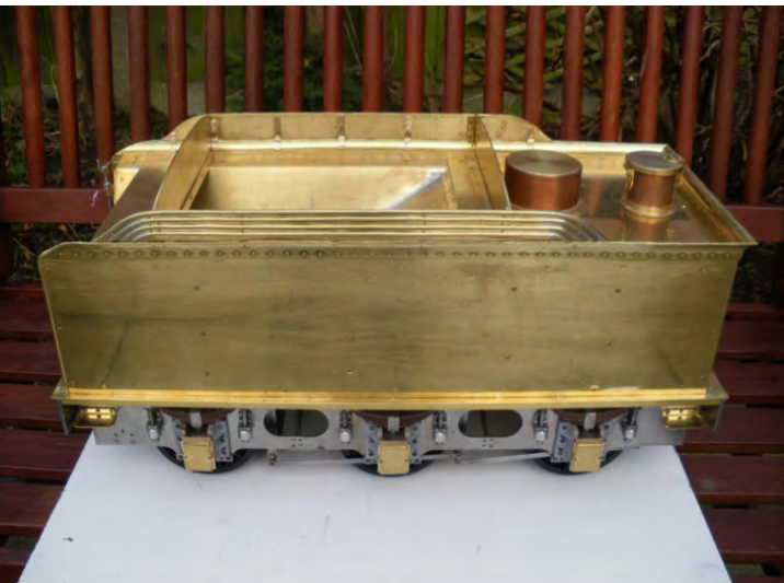
The tender tank ready for etching and final painting before final assembly. The frames still needed some work at this stage
