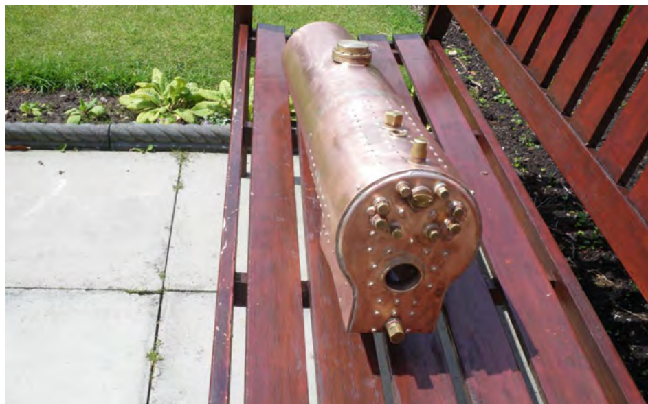
Boiler plugged in preparation for its hydraulic test
