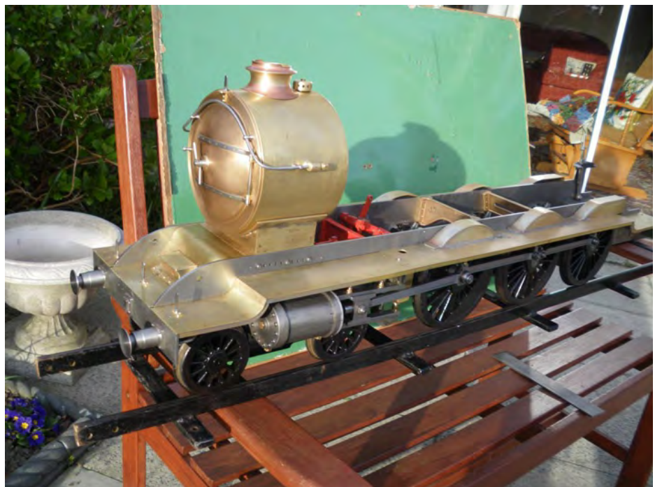
The final assembly of the Smokebox fittings with the Blast pipe and Petticoat pipe fitted
