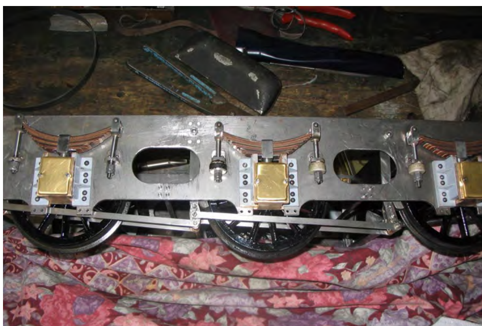
The tender frames in progress showing the leaf springs and compensated brake rigging
