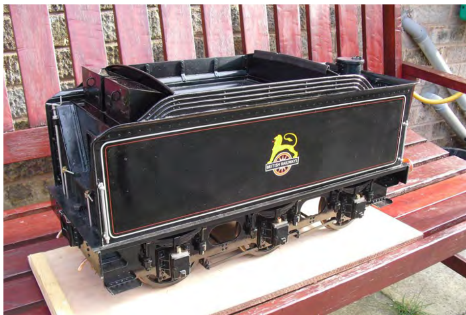
The tender tank ready for etching and final painting before final assembly. The frames still needed some work at this stage
