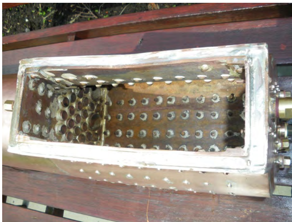
Boiler plugged in preparation for its hydraulic test
