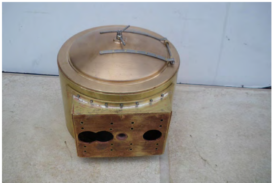
Steam fittings and Exhaust passages on the inside cylinder block
