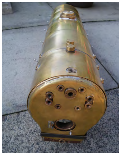
Trial fitting of the back-head cladding before final assembly
